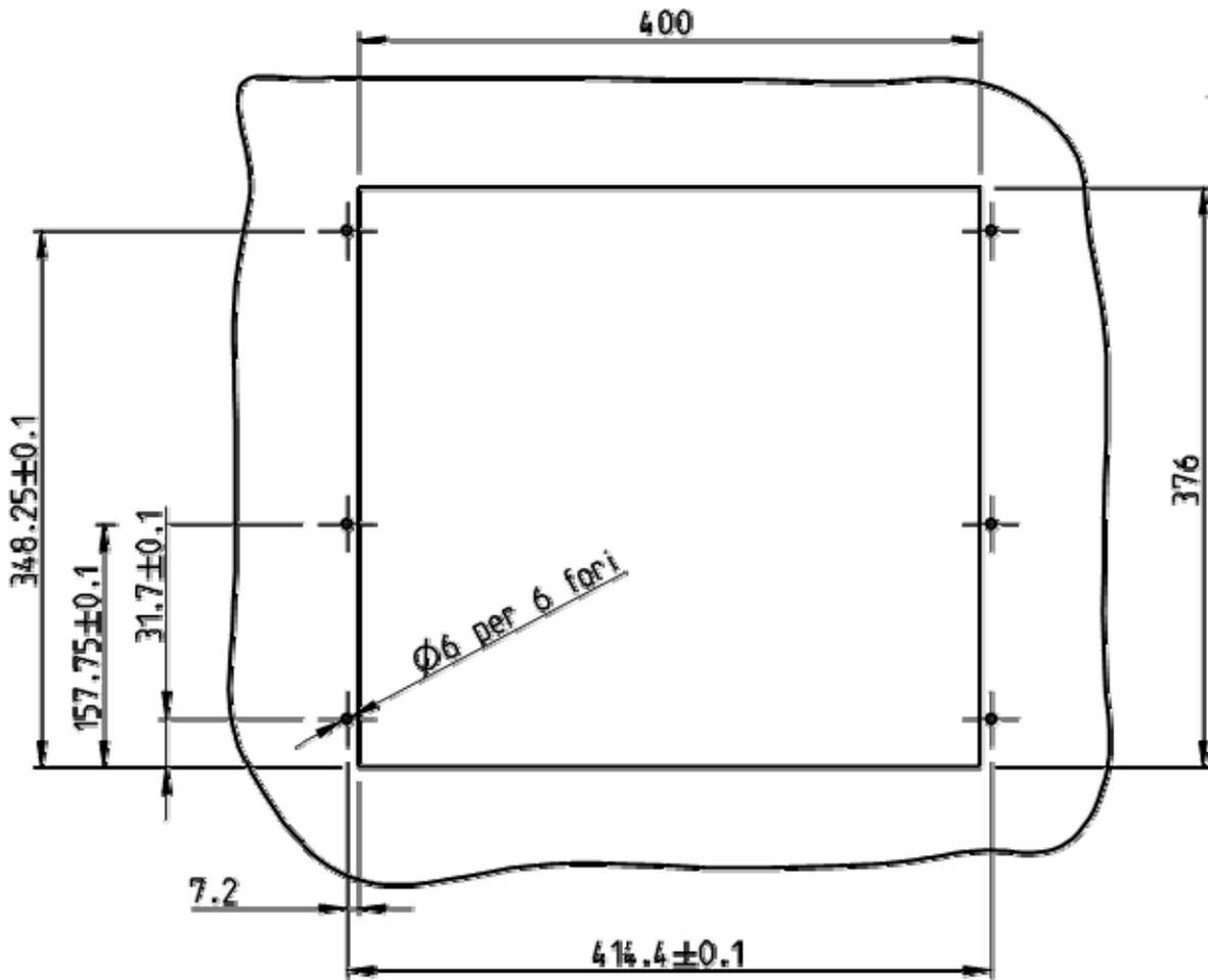
**Power D 15", 80 keys drilling template**
