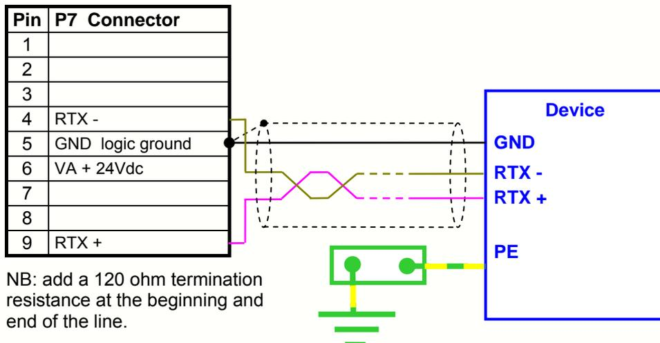
NB: add a 120 ohm termination resistance at the beginning and end of the line.
