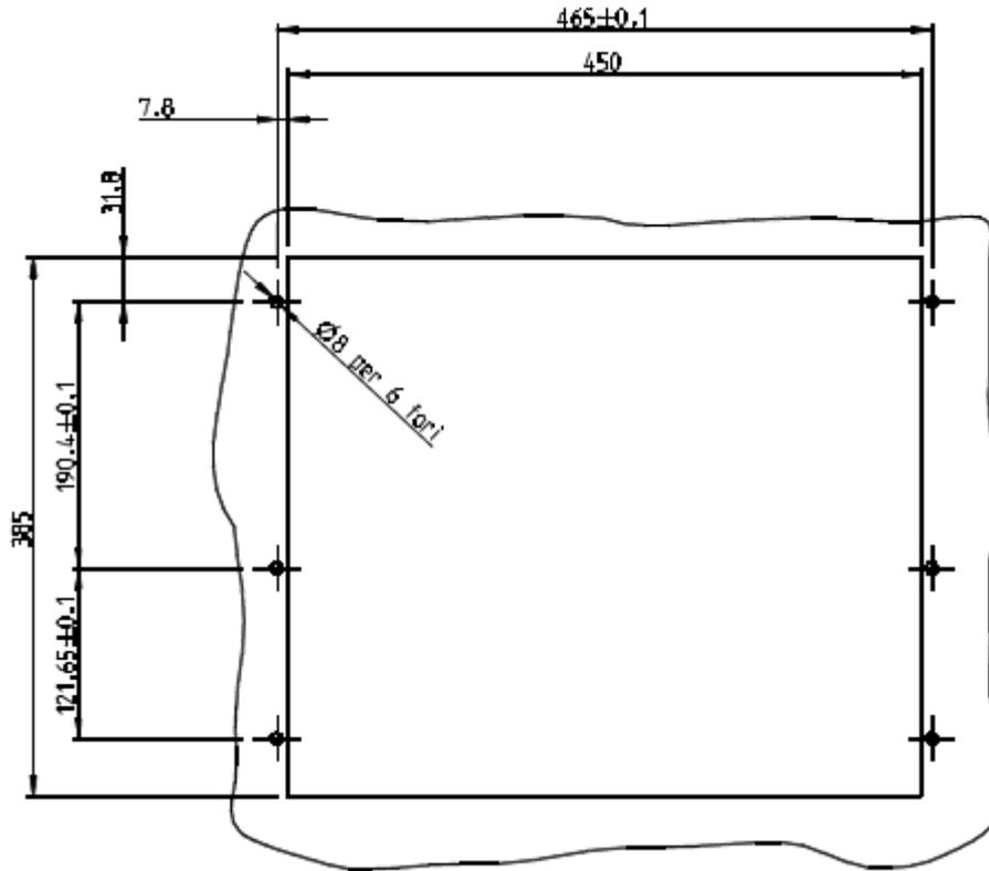
**Power D 15" - 28 keys drilling template**
